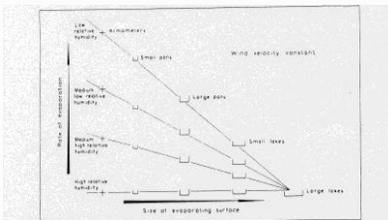
Figure 4.5. The relationship between the rate of evaporation, the size of the evaporating surface and the relative humidity. (From an original diagram by Thornthwaite and Mather, 1955).
