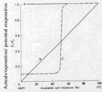
Figure 4.15 The relationship between actual and potential evaporation through the range of drying from field capacity (FC) and wilting point (WP) according to Penman and Monteith (line A), Thornthwaite (line B) and Panman (curve C). See text for explanation.
